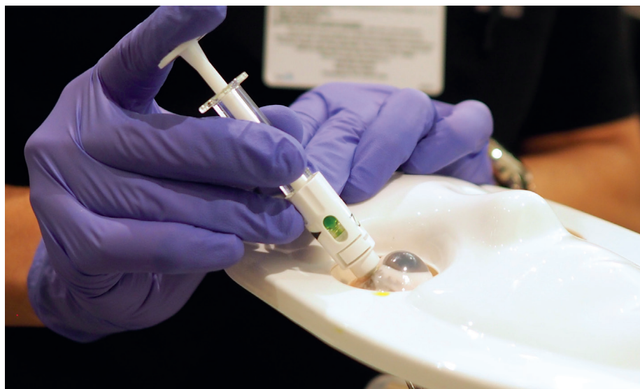
Figure 3: Demonstration of Suprachoroidal Advanceable Microneedle Device’s dial rotation feature to advance the needle while performing injection. Prototype design not available for sale or approved for use in any jurisdiction.
