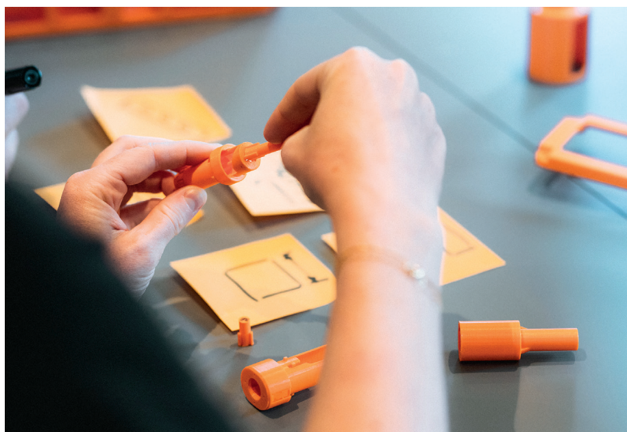
Figure 5: Hands-on evaluation of a device prototype with modular components – designing for easy disassembly supports more efficient recycling and sustainable end-of-life processing.
