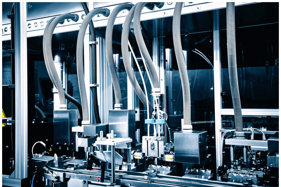
Figure 4: Testing pressure, tightness and flow.
