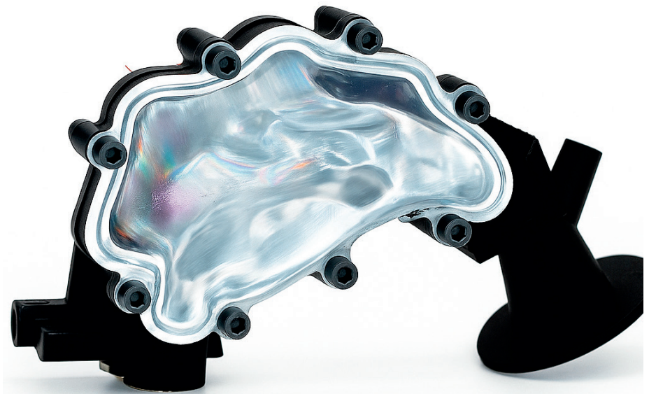
Figure 4: Anatomically representative human nasal passage airflow ducting used to quantify deposition patterns in experimental characterisation campaigns.
