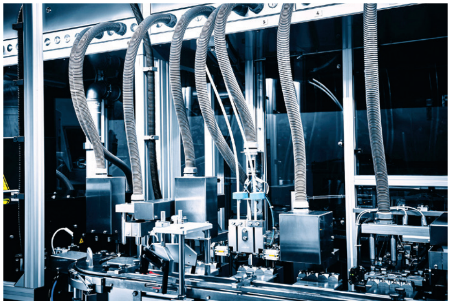
Figure 4: Testing pressure, tightness and flow.
