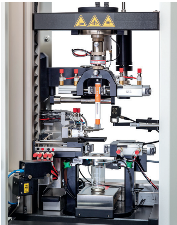
Figure 1: Example test setup according to ISO 11608-5. The test sequence combines multiple measurements within a single test.
