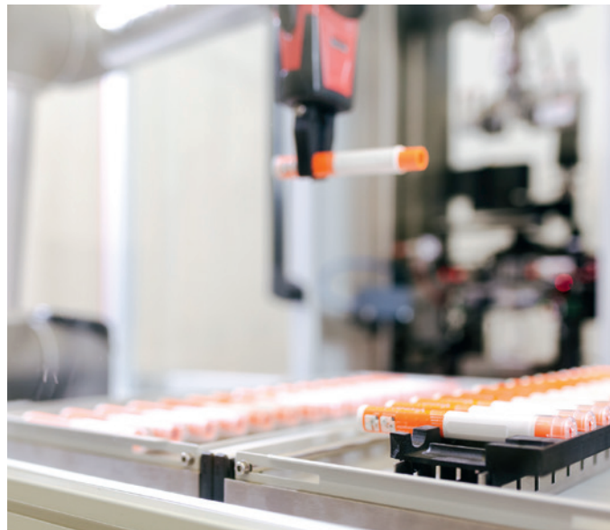
Figure 3: A fully automated testing system for autoinjectors.
