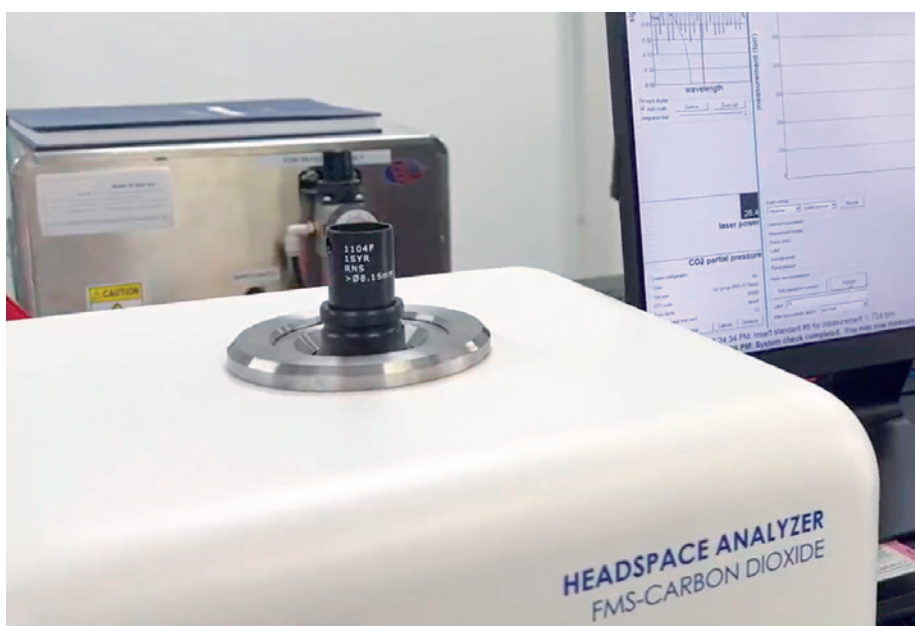
Figure 1: A laser headspace analyser at ZebraSci.
