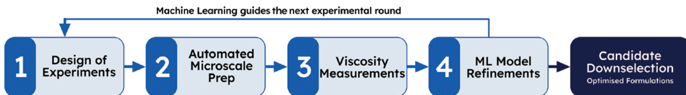
Figure 2: The AEMS iterative formulation workflow. Every experiment feeds a ML model that sharpens the next round of screening. Custom software automates the full cycle, from design of experiments through preparation, measurement and model update, enabling hundreds of experiments per week with minimal hands-on time.
