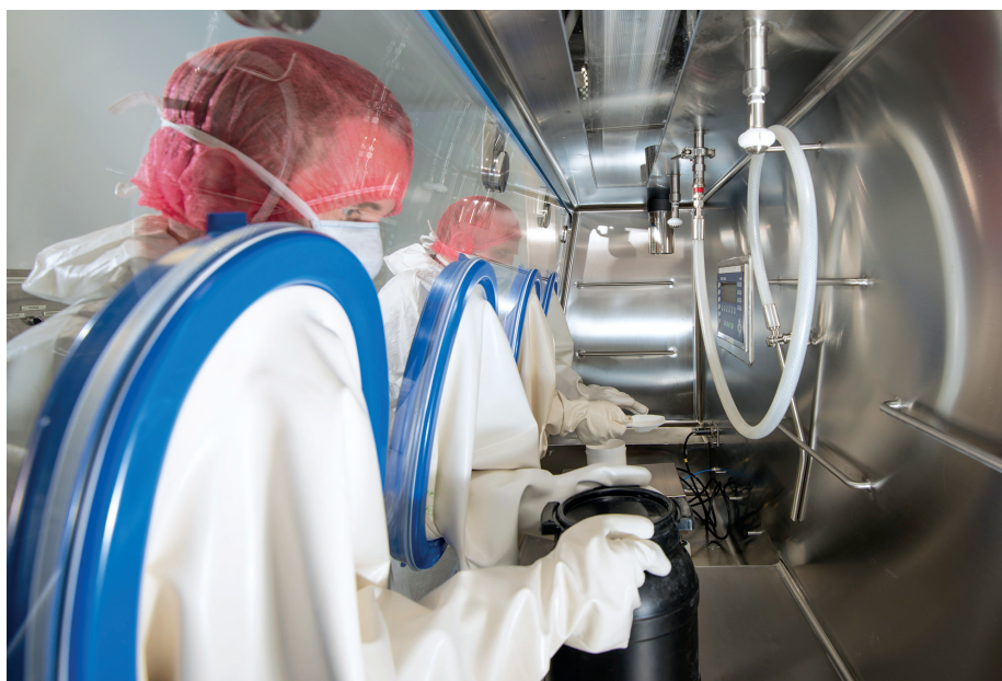
Figure 3: Interior of a manned high-potent isolator.
