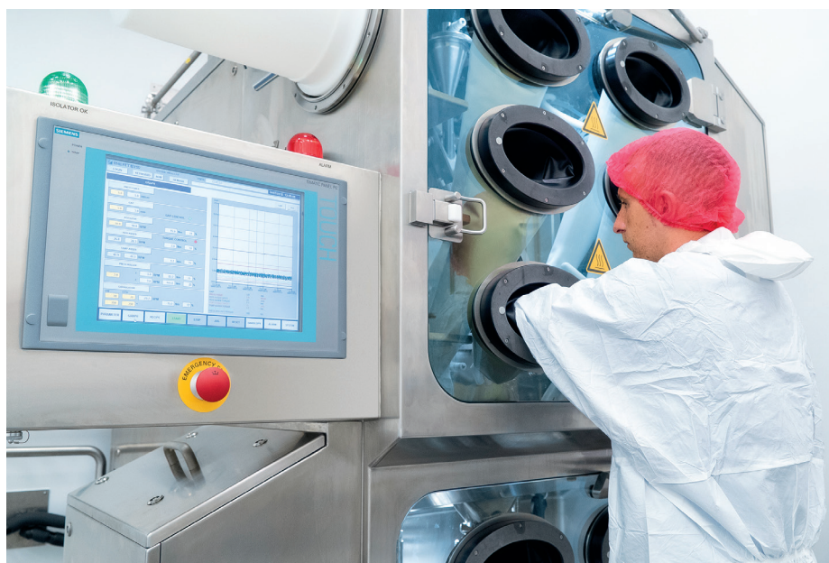
Figure 1: A Gerteis (Jona, Switzerland) roller compactor in use at PCI Pharma Services.
