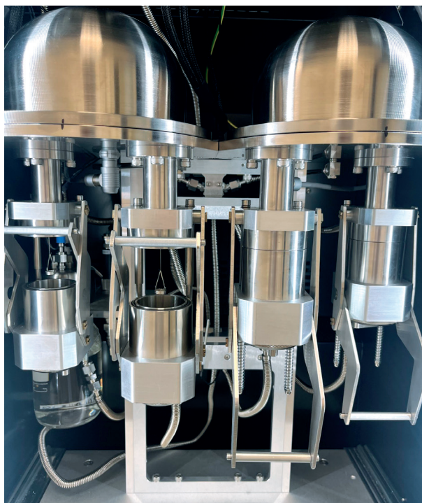
Figure 2: A DVS sample vessel used to determine mass changes in real time under varying humidity levels.
