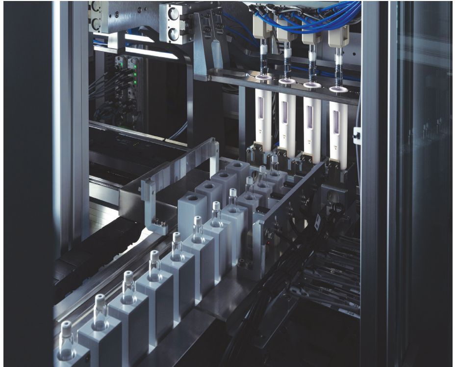
Figure 4: Interchangeable, project-specific puck carriers, fixtures and grippers on the transportation and assembly modules enable multidevice compatibility.
