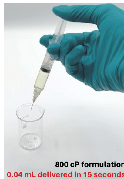
Figure 3: An 800 cP formulation is nearly impossible to inject via a standard 27G thin-wall needle. With 12% v/v saline sheathing fluid, CAF unlocks rapid injectability for the same formulation and needle. Here, the CO-AXL hub adapts disposable syringes for a vial presentation.
