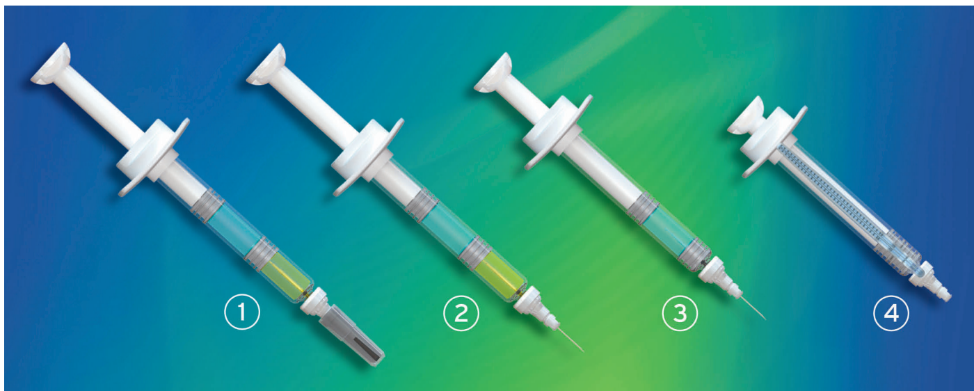
Figure 2: The Credence Sequential Dual Chamber system stores two liquids separately in the same standard PFS and allows the two liquids to be delivered with a single push of the plunger rod while also providing passive needle safety.
