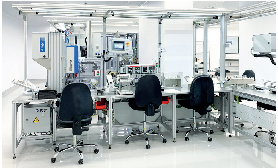
Figure 2: Manual workstation without carrier system.
