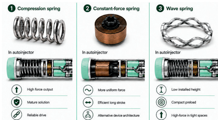
Figure 2: Choosing the right spring architecture – comparison of compression, constant-force and wave springs, highlighting how different spring types help designers manage force, stroke length, installed height and motion control.
