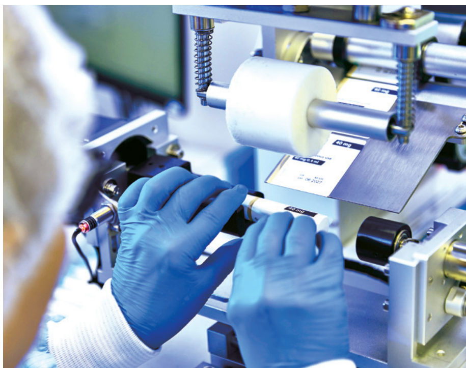
Figure 3: A platform autoinjector, being labelled on a semi-automatic labelling machine.
