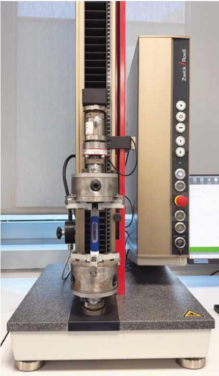
Figure 5: Cap removal force testing.
