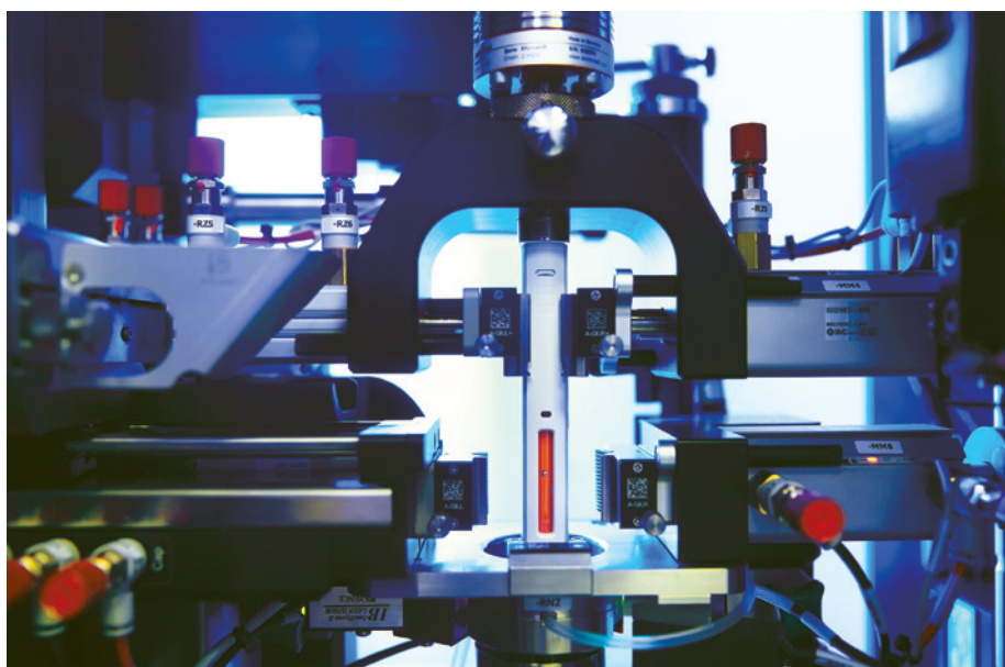
Figure 1: A platform autoinjector, undergoing functional testing on a ZwickRoell (Ulm, Germany) testing machine.
