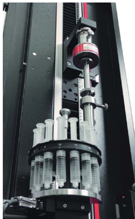
Figure 5: Rotary table system for high-precision testing of dose accuracy, breakaway force and glide force in syringes.
