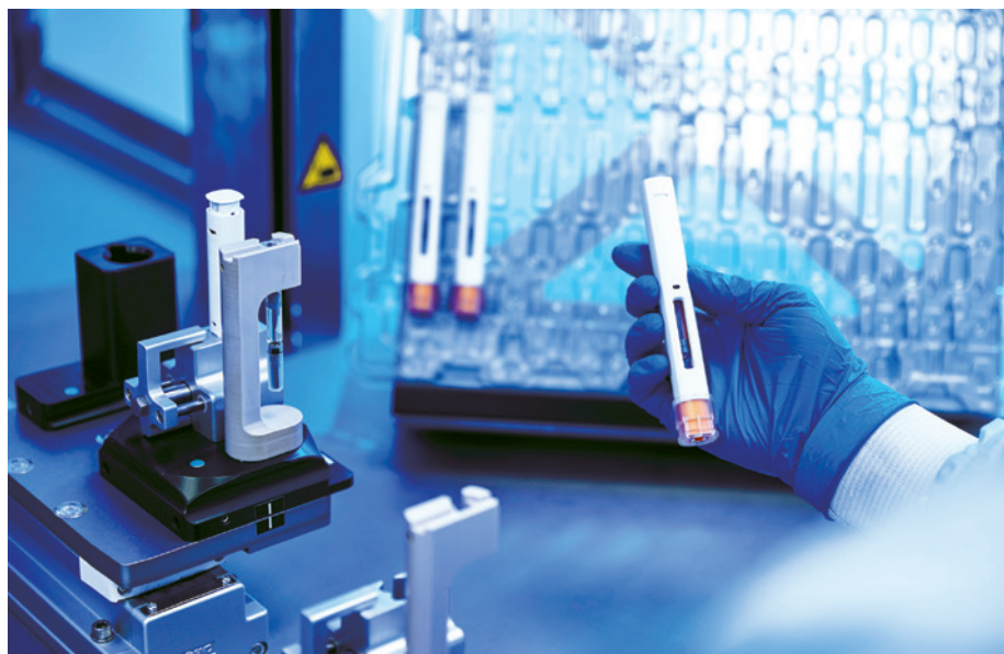
Figure 2: A platform autoinjector, following semi-automatic assembly on a Mikron (Neuchâtel, Switzerland) MAIA assembly machine.
