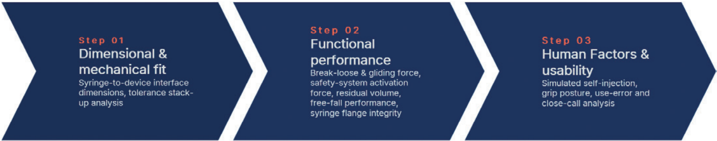
Figure 4: The joint SCHOTT Pharma–Nemera compatibility testing framework, from dimensional fit through functional performance to human factors usability.
