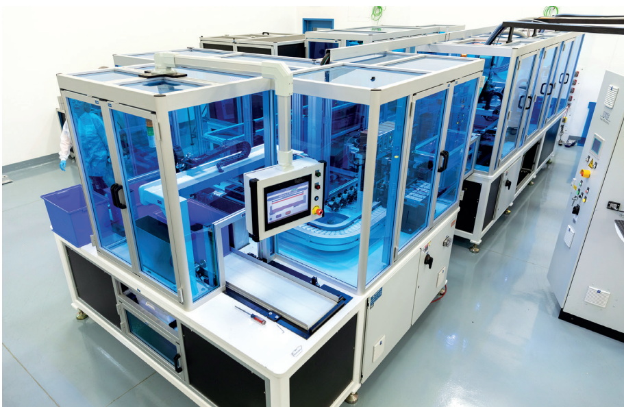
Figure 4: Automated assembly cells inspect and assemble device components with the precision, consistency and throughput required for commercial-scale manufacturing.
