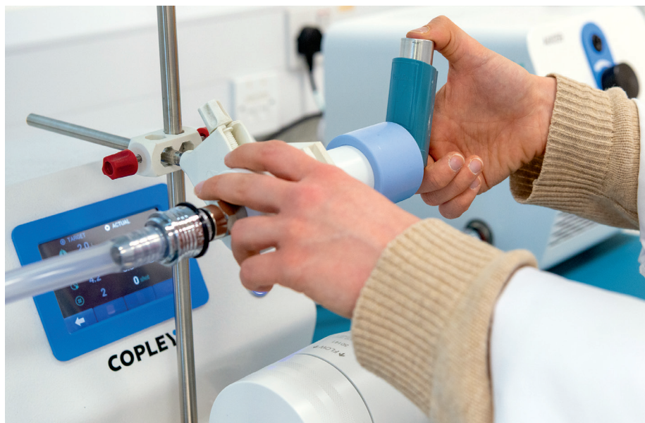
Figure 1: A dose-uniformity sampling apparatus for collecting delivered doses for delivered dose-uniformity testing.
