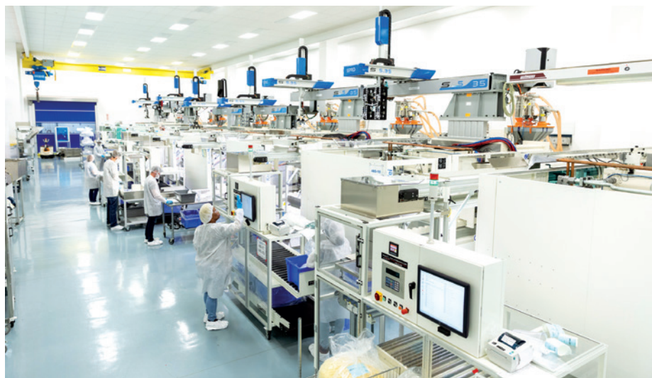
Figure 1: A commercial-scale production floor, where injection moulding and automated assembly bring device designs from development to high-volume manufacturing.
